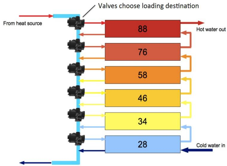
The charging "circuit" on the left is used to selectively heat up individual cells. The stack is shown here in a half-discharged state where the lower three cells have already crystallised.
