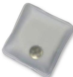
In the hand warmer above crystallisation is induced by flexing a metal disc that produces tiny metal particles. This intervention is enough to cause "nucleation" which sodium acetate in its normal state requires in order to crystallise. As it does so, the hand warmer becomes hot to touch until all its latent heat is given up and the solution has largely solidified. This produces enough heat to warm your hands for several minutes, after which the sodium acetate will be largely solidified.
